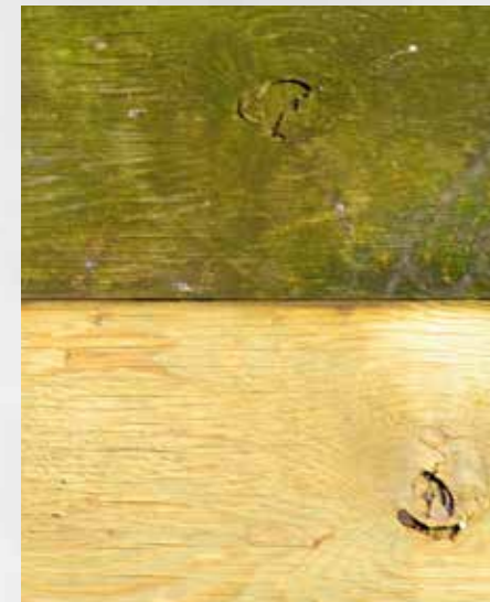
Before and after: APC with HydroBrite used to clean mold stained plywood.
